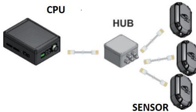
The maximum length of the connection depends on the supply voltage of the system and on the cross section of the UTP cable (AWG). For convenience, the reference tables of both connections will be provided.
