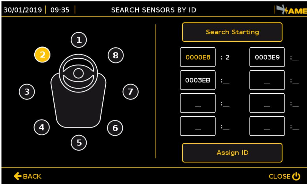
If the allocation procedure has been successful, the sensors turn green and the associated IDs move to the new positions. In case of error, try making the allocation again.
