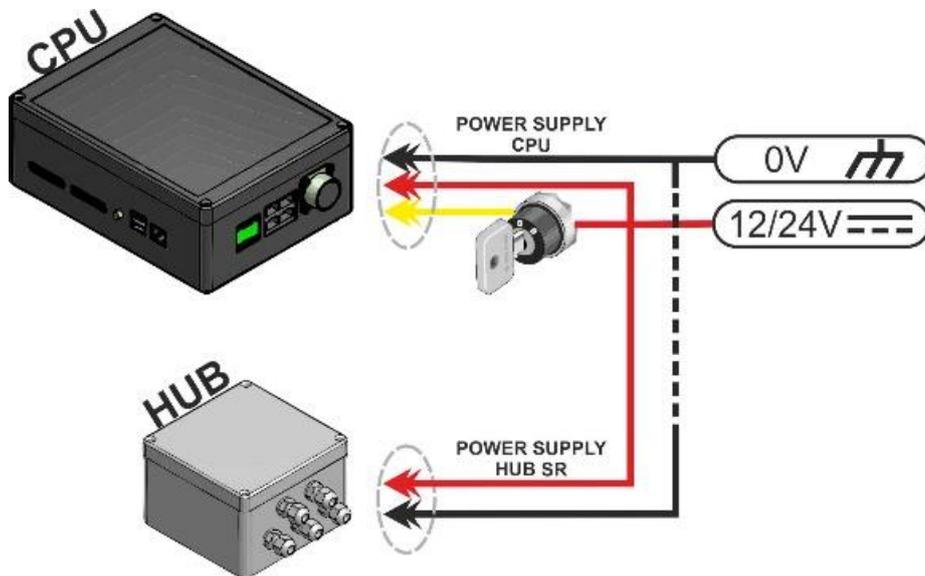
For the power supply connections, it is recommended to use an AWG 18 /0.75mm<sup>2</sup> cable or a cable with a higher cross section.
