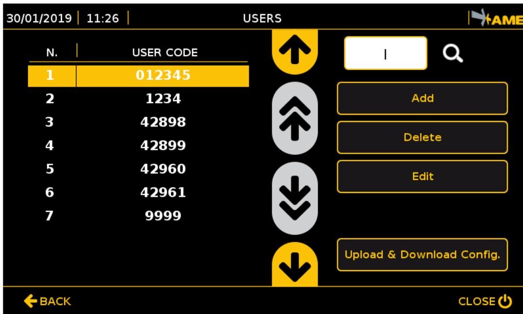
The Users section shows the codes of the Tags that were entered into the system master data for login and logout (paragraph 9.5).
