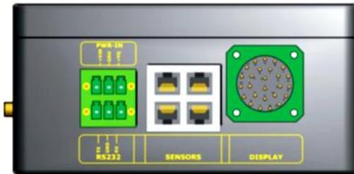
Power supply /turning-on RS 232      Sensors HUB (RJ45)      Display connector
