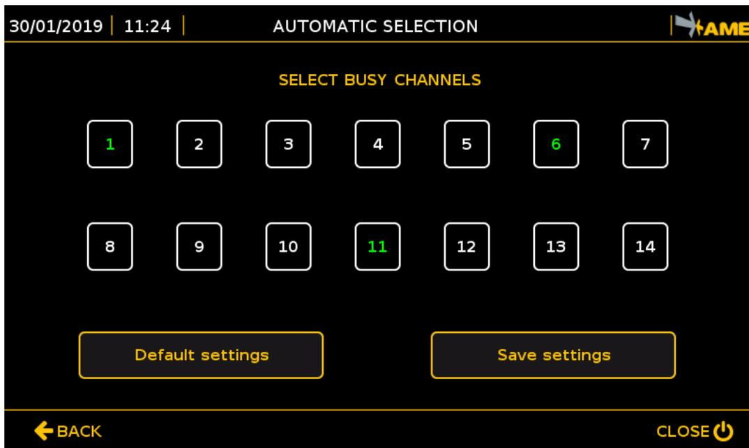
With the **Automatic Selection** mode, the operating frequency of the sensors is set automatically taking into account the channels, in the 2.45 GHz band, already taken by other systems that were entered into the section of the busy channels.
