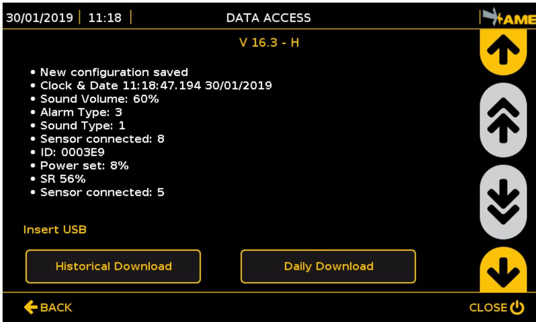
Press the key with the USB icon and enter the relative password to access the data page in which the history of events is shown.
