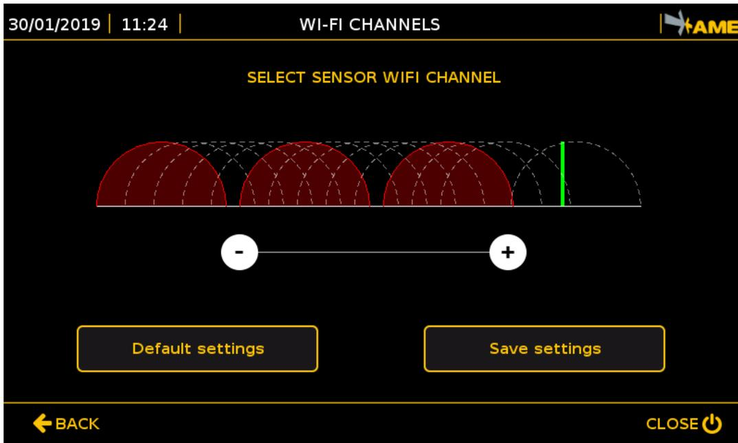
In manual mode, the operating frequency can be selected along the entire 2.45 GHz band no matter if the channels are busy or not.
