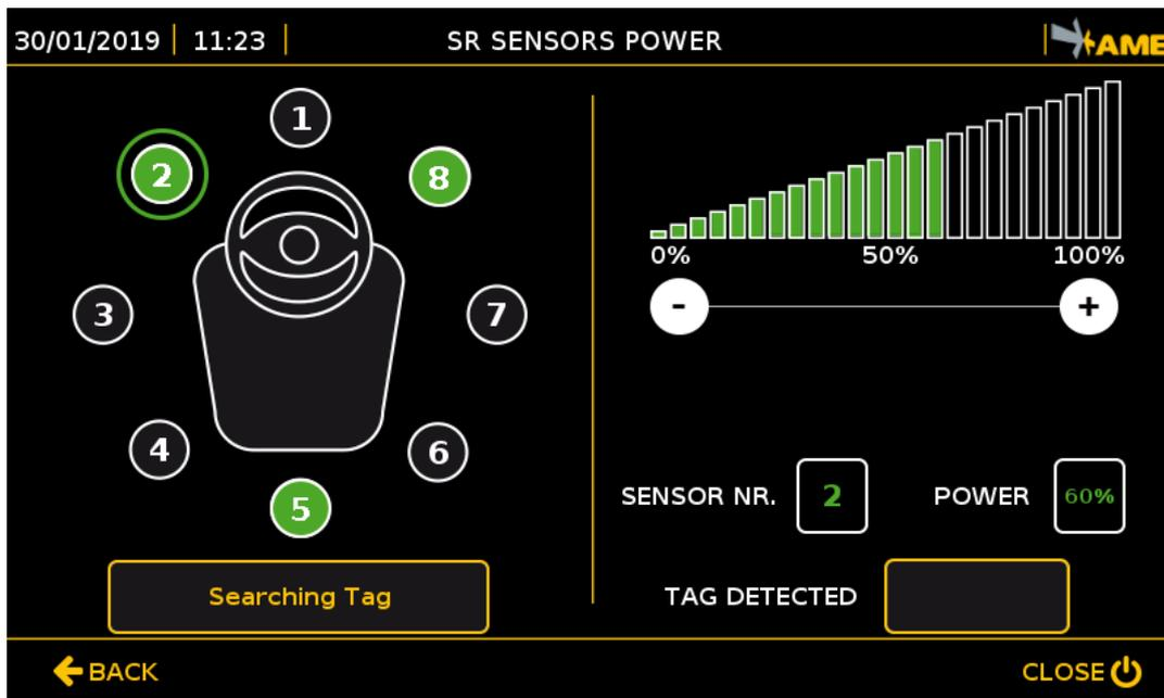
Adjust the SR sensor power to change the Tag, and so the pedestrian worker, detection distance in the Pre-Warning area.
