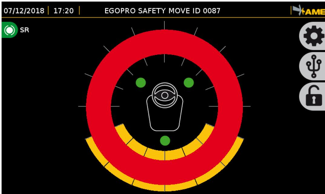
The presence of the pedestrian worker wearing an active TAG within the **WARNING** activation range is signalled to the driver via the display by means of a clearly visible red ring.
