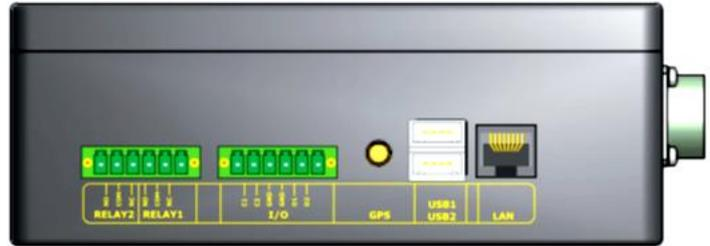
Relay      I/O      GPS Antenna      USB      LAN
