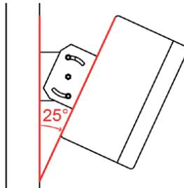
NOTE: the mechanical joint supplied can be used to obtain the desired inclination.
