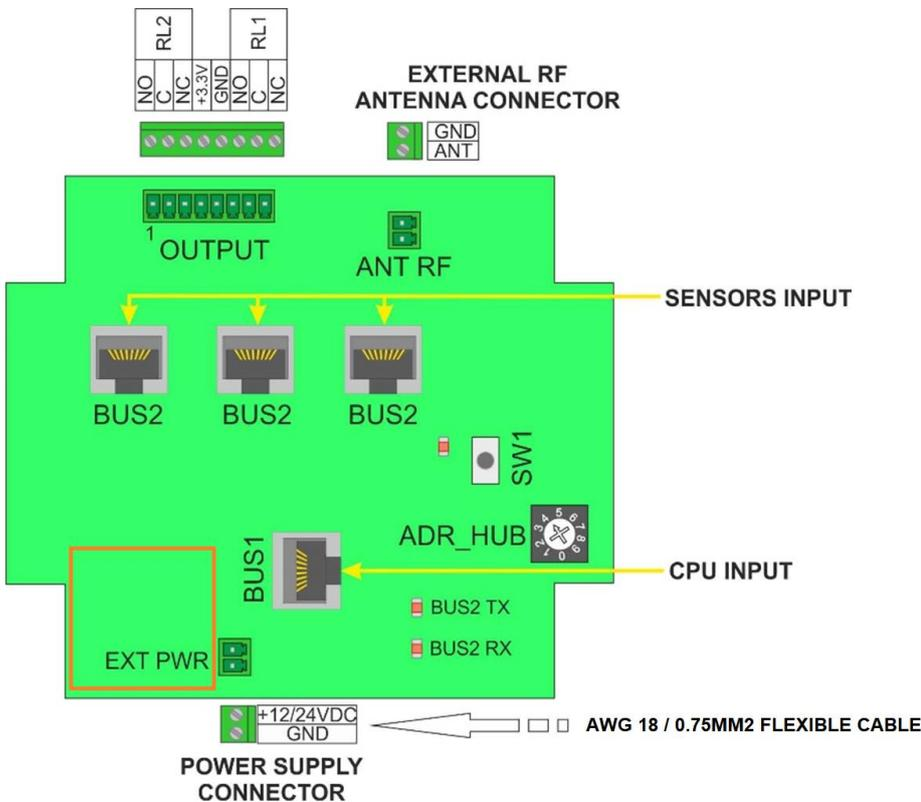
We recommend to keep the coaxial antenna cable far from the zone marked with the orange square.
