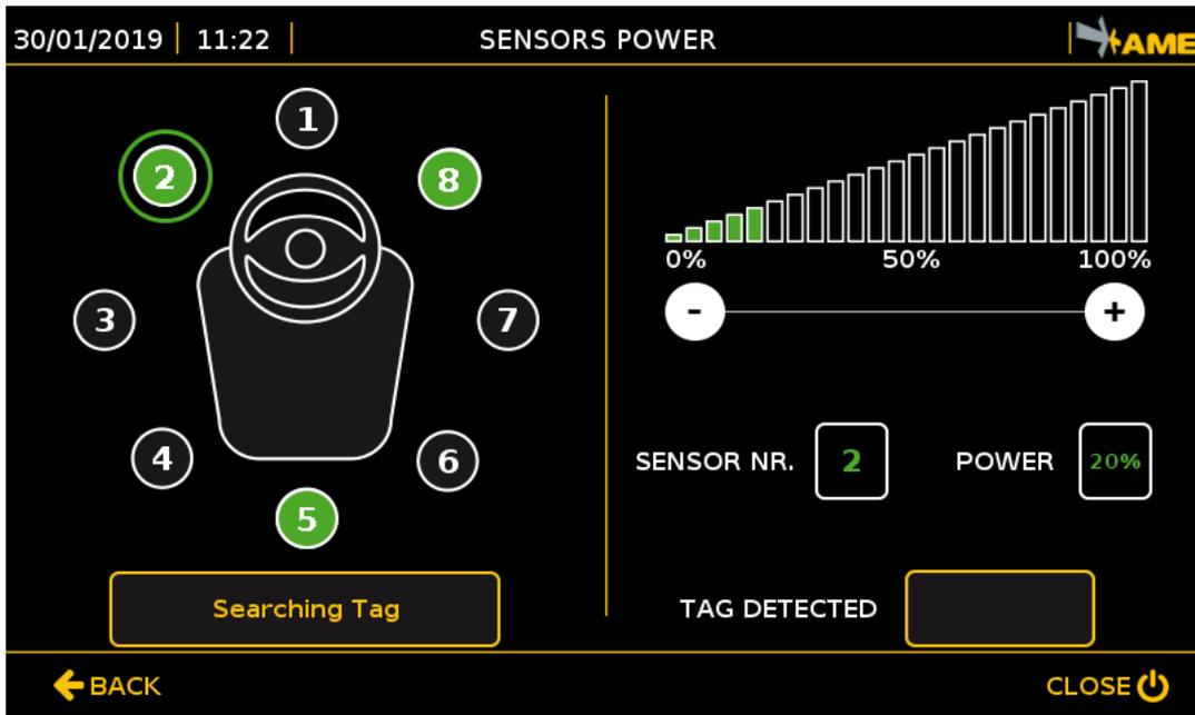
Adjust the LR sensor power to change the Tag, and so the pedestrian worker, detection distance in the Pre-Warning area.
