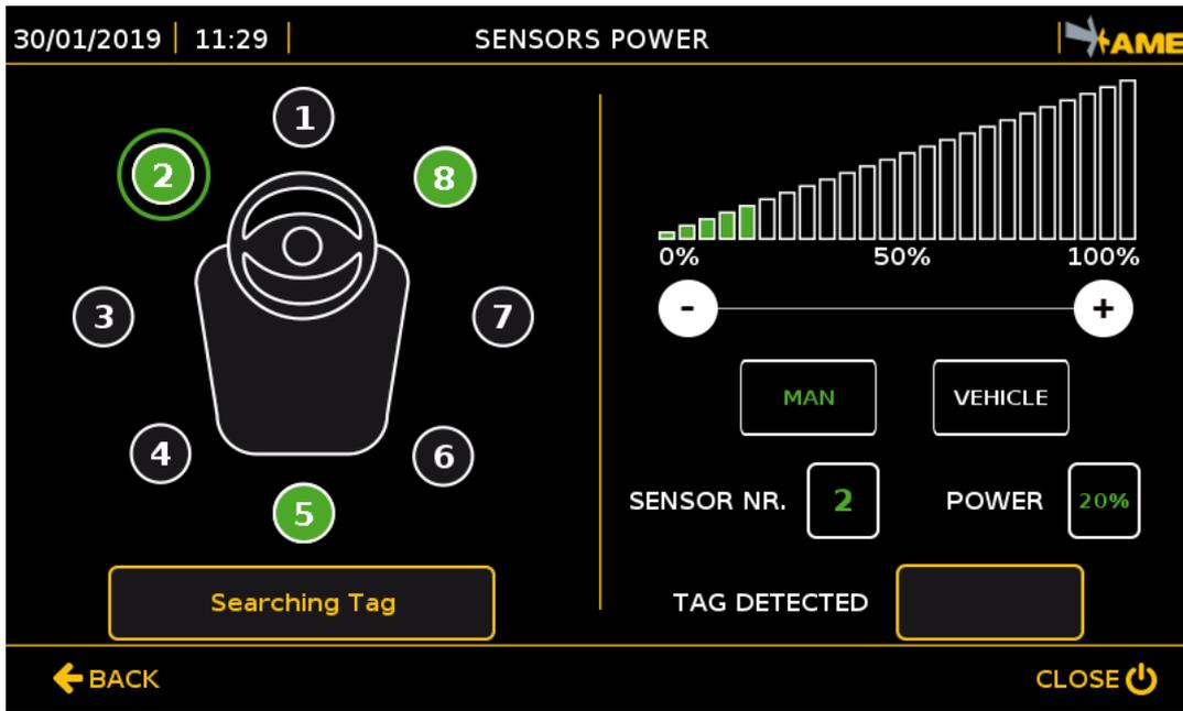
In this section, the sensor power, and thus the detection distance of both the pedestrian worker’s Tag and the vehicle’s Tag, can be changed.
