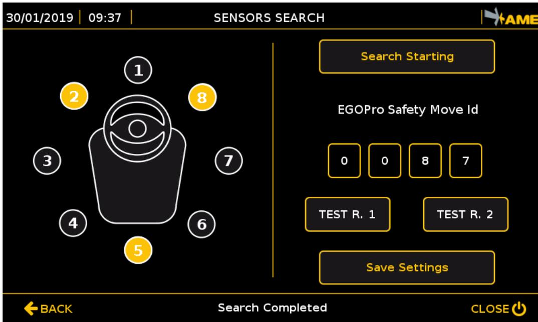
If the ID search has been correctly performed, the selected sensors (e.g. 2, 5 and 8) will turn yellow. Press the SAVE SETTINGS key: the colour of the sensors will change from *yellow* to *green*, and, as of that moment, the sensors will be associated to the vehicle.
