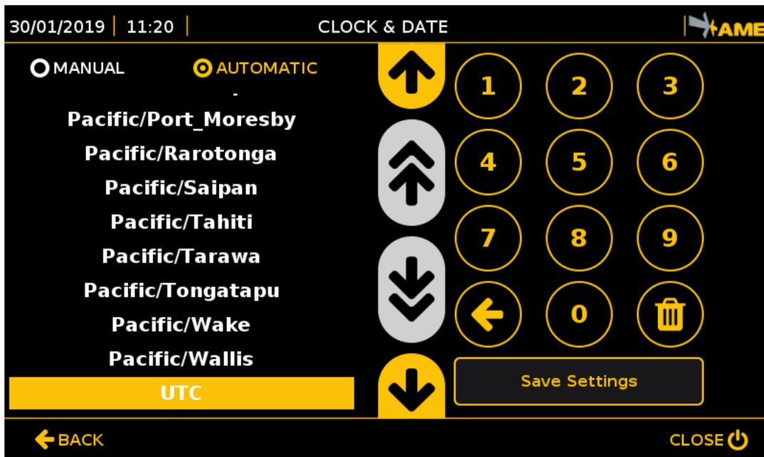
In automatic mode, the internal clock of the system becomes automatically synchronised by means of the network (if available) or the GPS module if installed.
