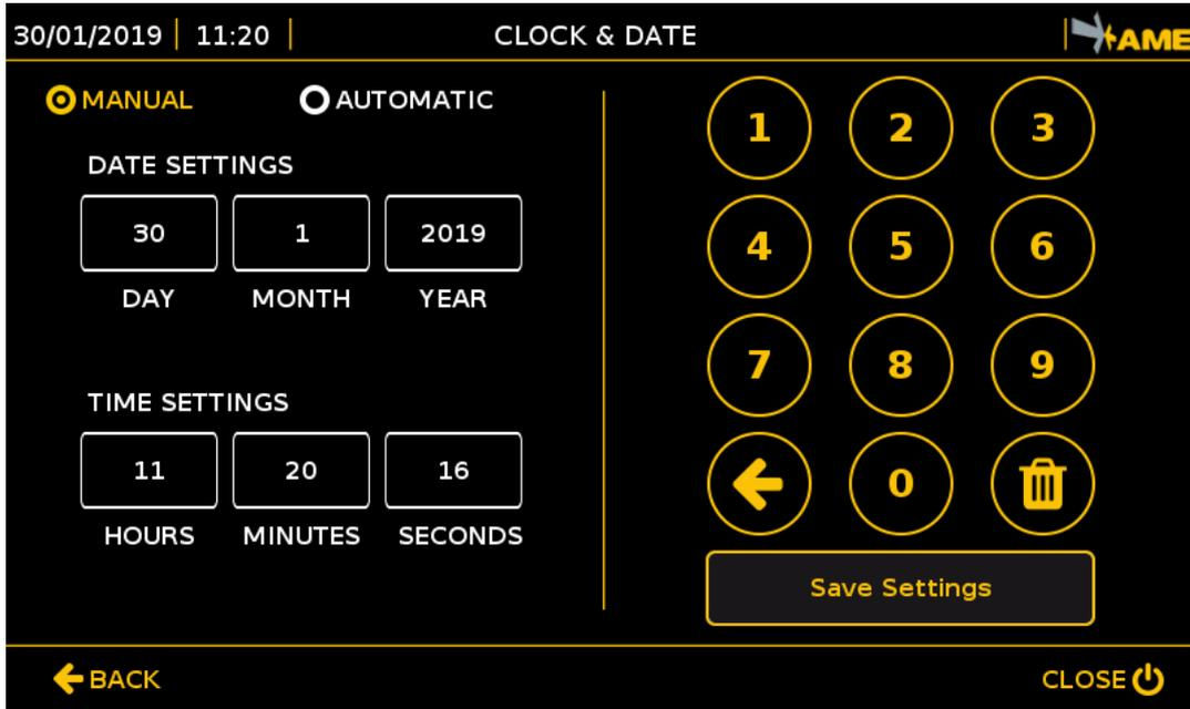
In manual mode, the internal clock of the system must be set by filling in all the fields manually.
