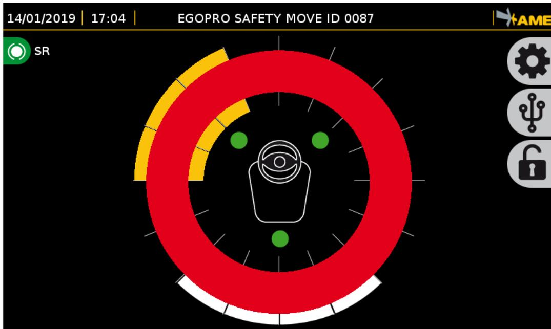
The vehicle-vehicle proximity warning module detects not only the pedestrian worker moving around the vehicle, but also other vehicles equipped with the specific EGOpro Safe MOVE sensors.
