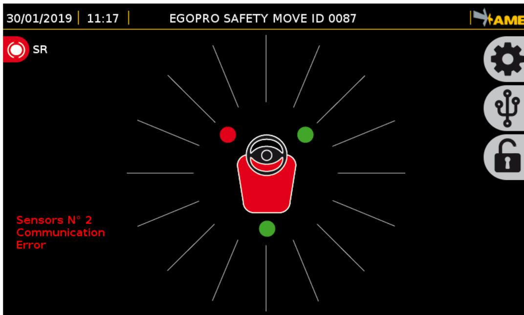
Active sensors are displayed matching their position on the vehicle. Only installed and configured sensors are shown on the display.
