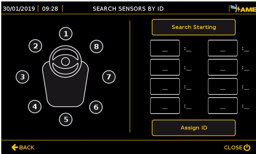
Press the SEARCH STARTING key to display all the sensors connected to the system.
