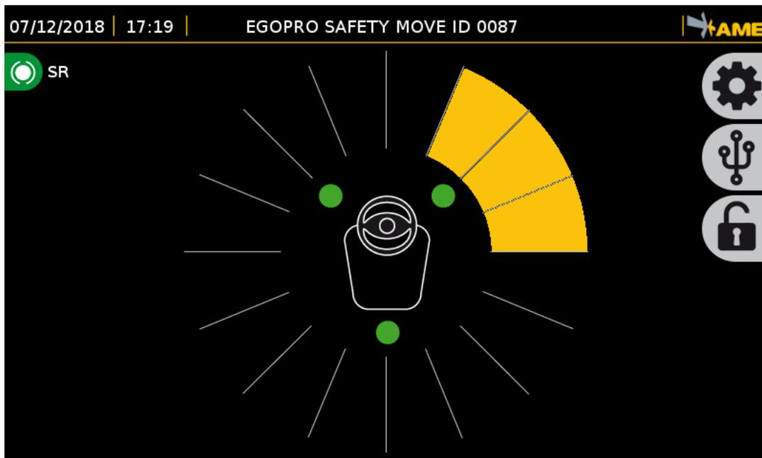
The presence of the pedestrian worker wearing an active TAG within the **PRE-WARNING** activation range is signalled to the driver via the display that shows the position of the pedestrian worker around the vehicle.
