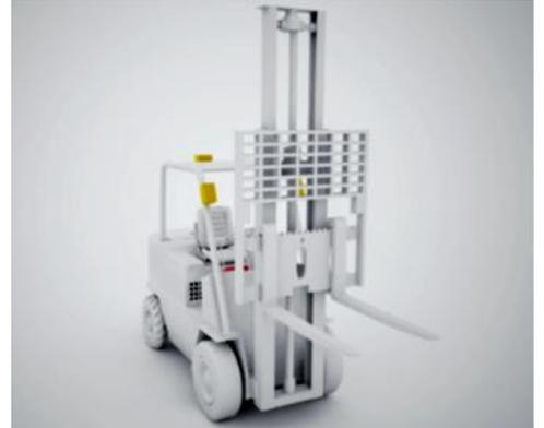
The sensors must be positioned on the perimeter of the vehicle in order to have maximum visibility between Sensors and TAG. On small/medium-sized vehicles, they are usually positioned on the uprights immediately below the roof and with a 25 ° downward inclination.
