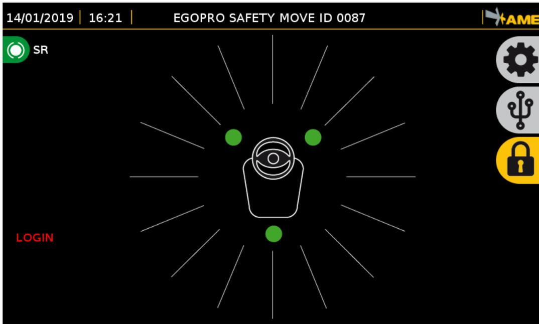
The LOGIN operation is used to check which operator is driving the vehicle at the date and time requested, and it is essential to exclude the driver’s TAG from the Proximity Warning & Alert System. When the system is turned on, the main interface presents a lateral red message inviting the user to LOGIN, which is signalled by a yellow icon.
