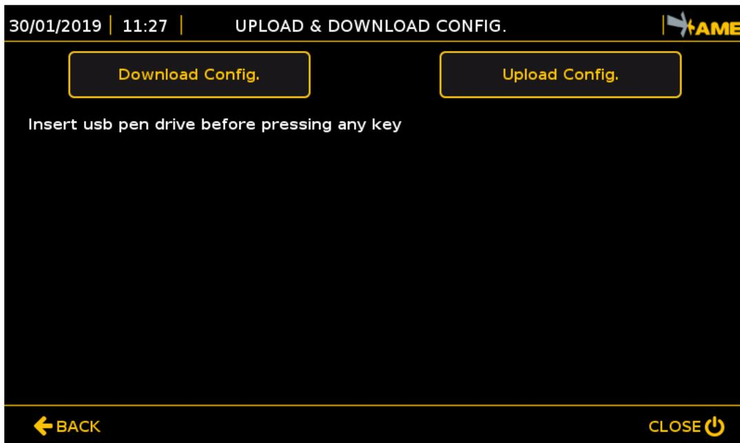
All users can be configured in a system, and then, by means of these functions, the list of users can be copied to the remaining systems without having to enter the users in all vehicles manually.
