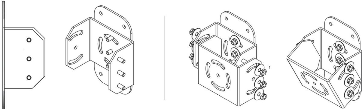
Find below the heights for the possible holes to be used for fixing it to the plate.
